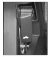
2. Pull the handle located on the lower part of the instrument panel.
